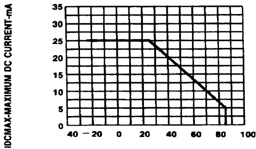
Fig.4 MAXIMUM ALLOWABLE DC CURRENT PER SEGMENT VS. A FUNCTION OF AMBIENT TEMPERATURE.
